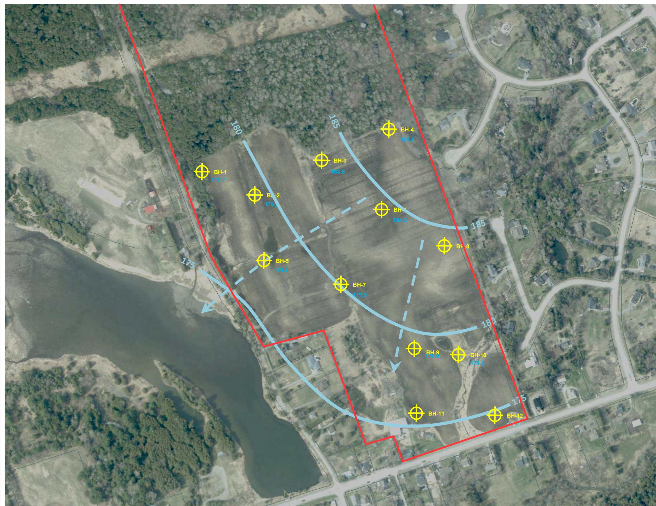
FIGURE 3: SITE PLAN SHOWING SHALLOW GROUNDWATER FLOW DIRECTIONS
