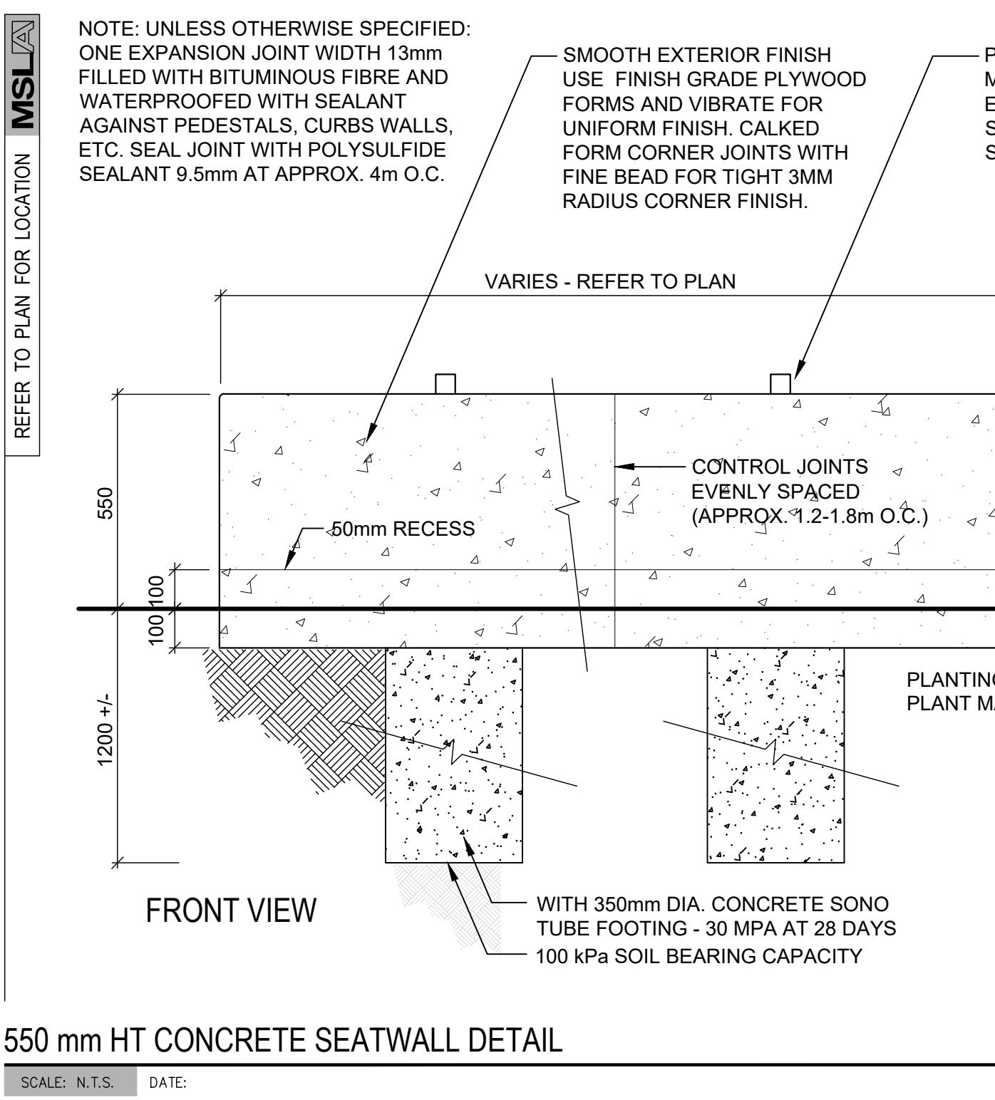
550 mm HT CONCRETE SEATWALL DETAIL
