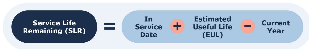
Figure 7 Service Life Remaining Equation
